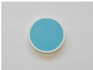
Figure 16: Pressed pellet with a layer of sample
