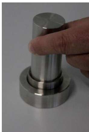
Figure 19: Placement of the pestle
