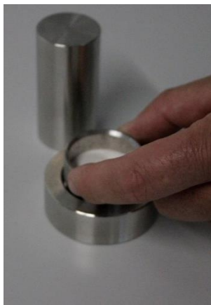
Figure 18: Place the ring in the tool
