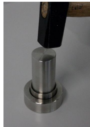
Figure 20: Knock out the sample with a hammer
