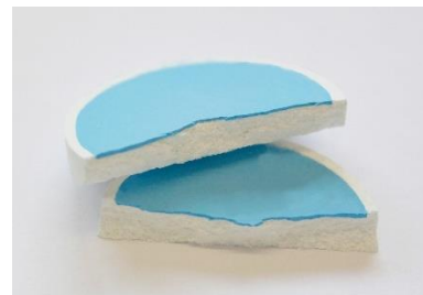
Figure 17: Breaking the sample shows the thin layer
