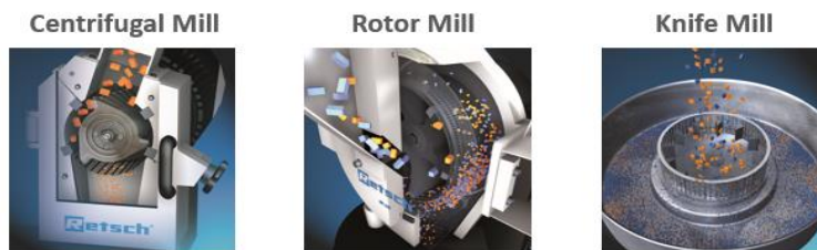
Figure 2 Principle: Grinding a sample
